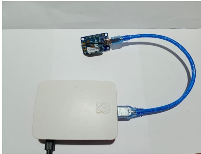
Rangkaian penerima data (Raspberry pi, Xbee Pro S2C dan Xbee adaptor)
