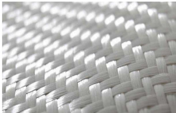
Gambar 4. *GFRP (Glass fiber reinforce polymer) sheet*
