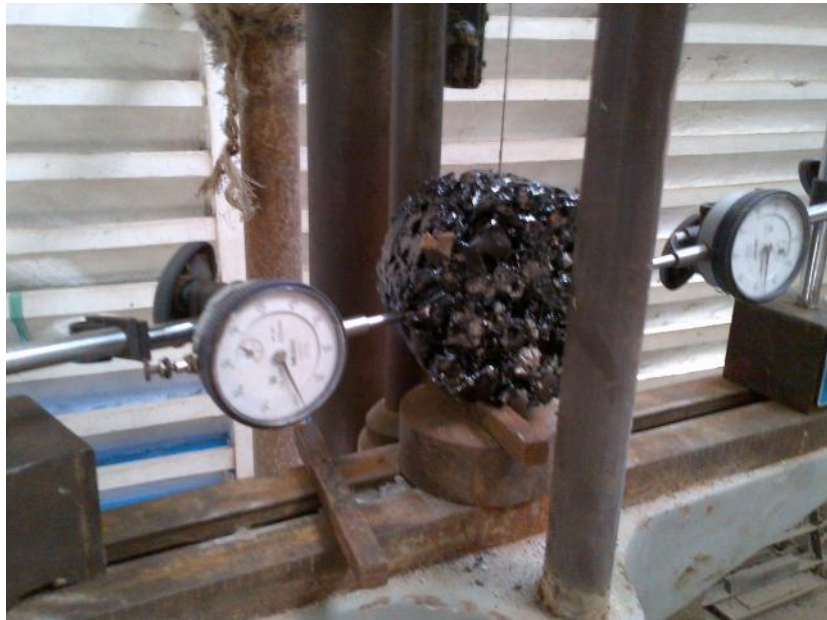
Gambar 32. Sampel Hasil Pengujian ITS
