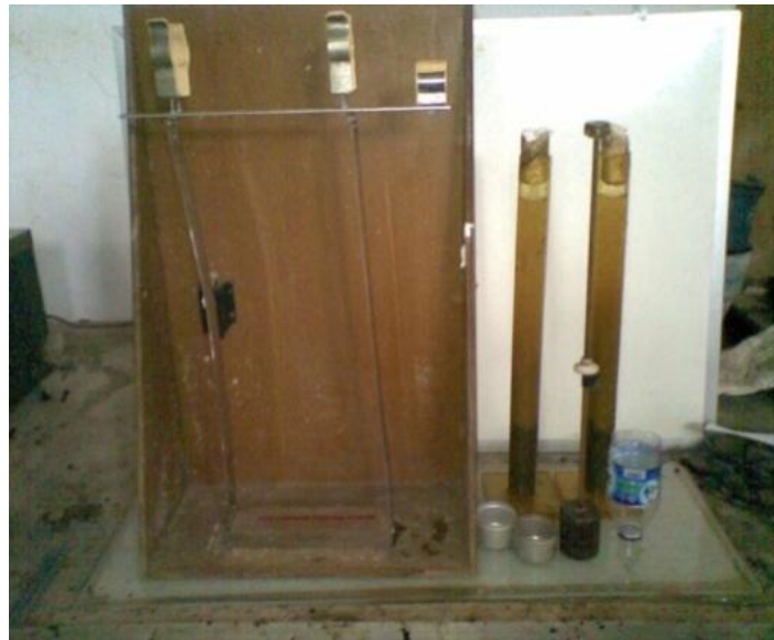
Gambar 11. Pengujian Kadar Lumpur Pasir ( Sand Equivalent Test )
