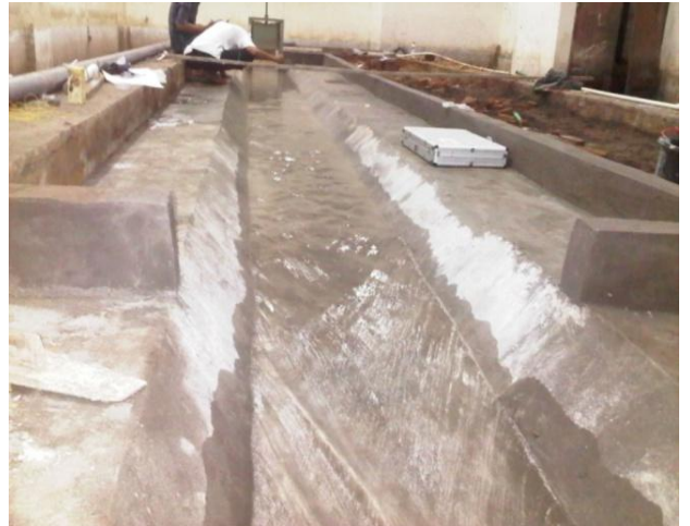
Percobaan running debit normal
