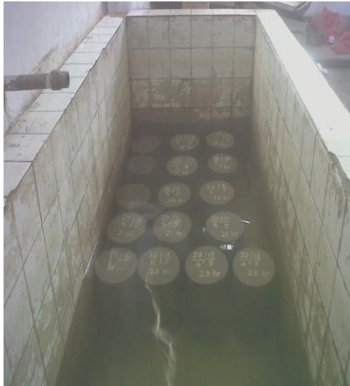
Gambar 26. water curing beton biotek Semen
