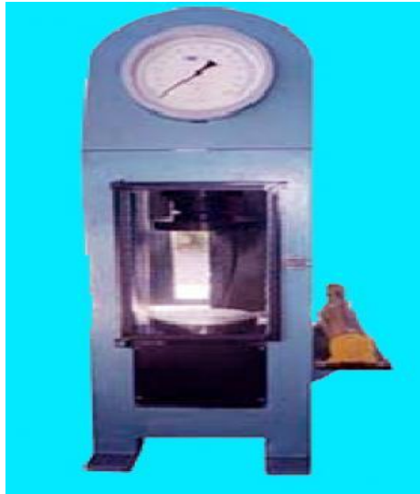
Gambar 8. Tampak Mesin Uji Tekan Beton (Compressive Strength Machine)
