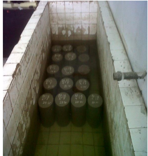
Gambar 27. water curing beton semen pcc
